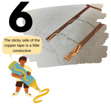
After that stick the LEDs legs down with the left over bits of copper tape.
