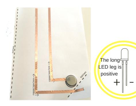
**4. ADD THE BATTERY** Put the battery + side down on the circle. Fold the corner upwards and secure it with a clip.
